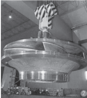
(a) Water TG unit for high-head pumped, storage power station (360 MW, 50 Hz, 12 poles, 500 rpm)
